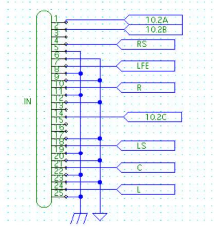
drawing relate to connections made between two units to support 10.2 channel bass management.
